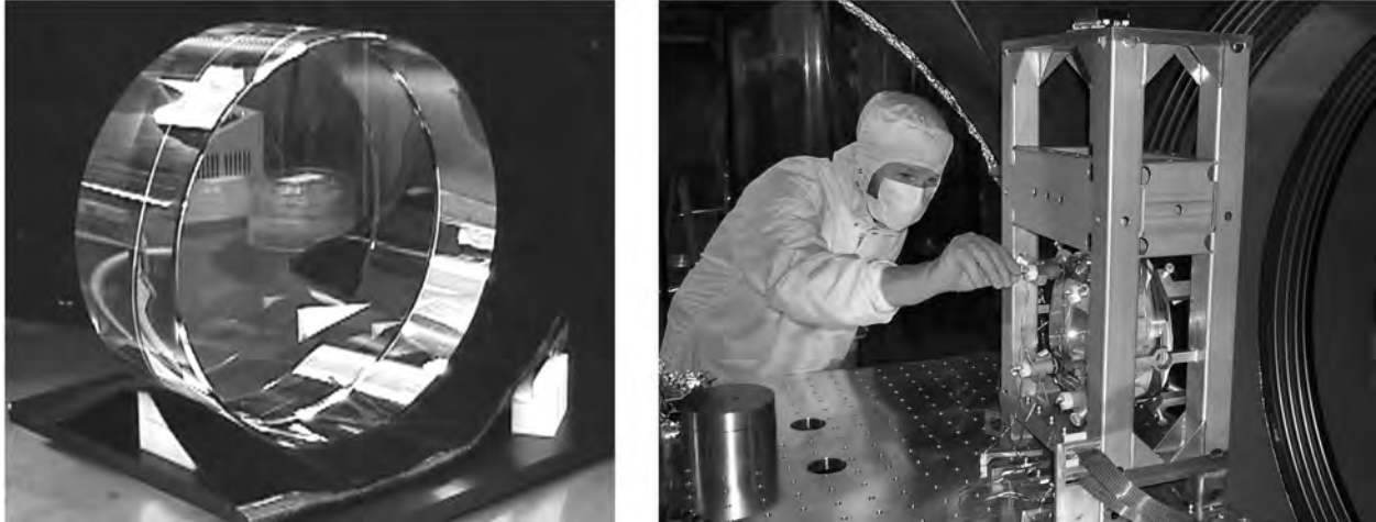
Figure 16: Left: A mirror for the initial LIGO interferometers, resting on a velvet cushion. Right: The mirror being hung by wires in its cradle in LIGO. [Courtesy LIGO Project, California Institute of Technology.]
