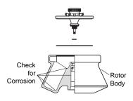
Periodically (at least monthly) inspect the rotor body for rough spots or pitting, white powder deposits—frequently aluminum oxide—or heavy discoloration. If any of these signs are evident, do not use the rotor. Contact your Beckman Coulter representative for information about the Field Rotor Inspection Program (FRIP) and the rotor repair center.
