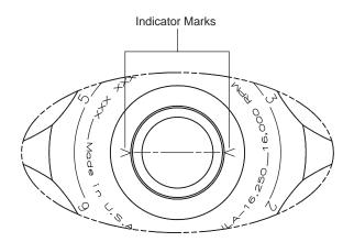
Figure 3. Rotor Top View: Indicator Marks Show Drive Pin Orientation
